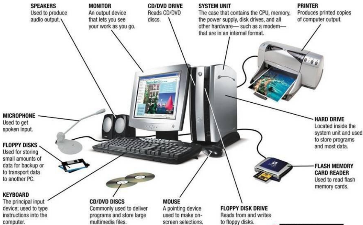
FIGURE 1-7 Typical computer hardware.
